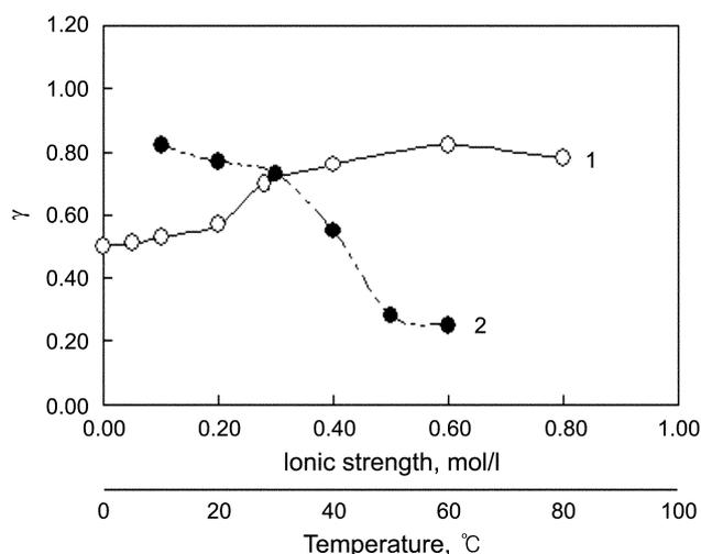
**Figure 5.** Effect of the operation conditions on  $\gamma$  of the solutions containing 1.0  $\mu\text{mol}$  IC/25 mL and 1.00  $\mu\text{mol}$  CTAB/25 mL: 1- ionic strength and 2- temperature.
