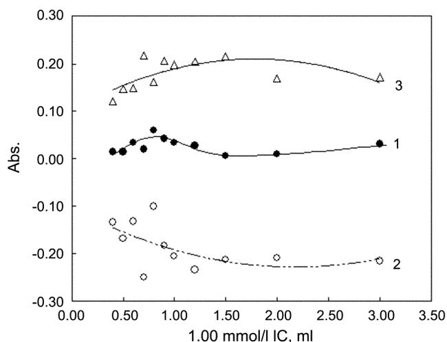
**Figure 6.** Effect of IC on the absorbance of the solutions containing 0.500  $\mu\text{mol}$  CTAB/25 mL: 1- measured against reagent blank at 560 nm, 2- same as 1 but at 610 nm and 3- calculated  $A_c$ .
