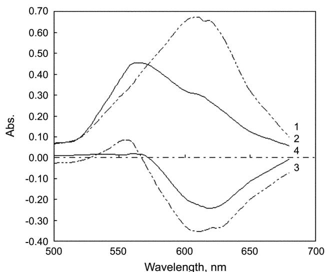
**Figure 3.** Absorption spectra of IC and its CTAB solutions containing 0.6 mol/L NaCl: 1- IC (1.00  $\mu\text{mol}/25\text{ mL}$ ) solution against water, 2- IC (1.00  $\mu\text{mol}/25\text{ mL}$ ) - CTAB (10  $\mu\text{mol}/25\text{ mL}$ ) solution against water, which does not contain free IC, 3- IC (1.00  $\mu\text{mol}/25\text{ mL}$ ) - CTAB (1.00  $\mu\text{mol}/25\text{ mL}$ ) solution against a reagent blank and 4- same as 3 but in absence of NaCl.
