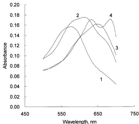
Fig. 3 Absorption spectra, recorded at room temperature, of CSTDD, Cu-CSTDD complex, Co-CSTDD complex and Cu-CSTDD-Co binuclear complex in corresponding solutions containing: (1) 0.01435 mmol/l CSTDD; (2) 0.01435 mmol/l Cu(CSTDD); (3) 3.00 mg/l Co(II) and 0.01435 mmol/l CSTDD, and (4) 0.01435 mmol/l Cu(CSTDD) and 3.00 mg/l Co(II) at pH 9.43.
