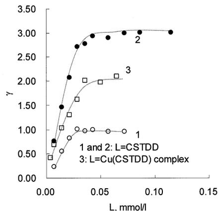
Fig. 5 Variation of  $\gamma$  with CSTDD and Cu(CSTDD) complex molarity in the corresponding solutions: (1) 1.00  $\mu\text{g/ml}$  Cu(II), L = CSTDD; (2) 1.00  $\mu\text{g/ml}$  Co, L = CSTDD and (3) 0.400  $\mu\text{g/ml}$  Co(II), L = Cu(CSTDD) complex.
