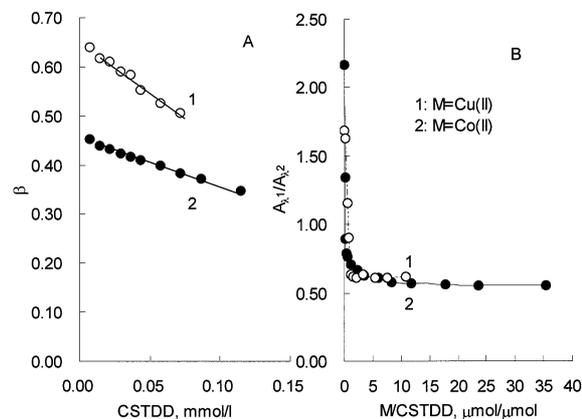
Fig. 2 (A) Variation of  $\beta$  with CSTDD molarity, (B) variation of the absorbance ratio of (1) Cu-CSTDD with the molar ratio of Cu ( $M = \text{Cu(II)}$ ) to CSTDD at pH 9.43, (2) Co-CSTDD with the molar ratio of Co ( $M = \text{Co(II)}$ ) to CSTDD at pH 9.43.
