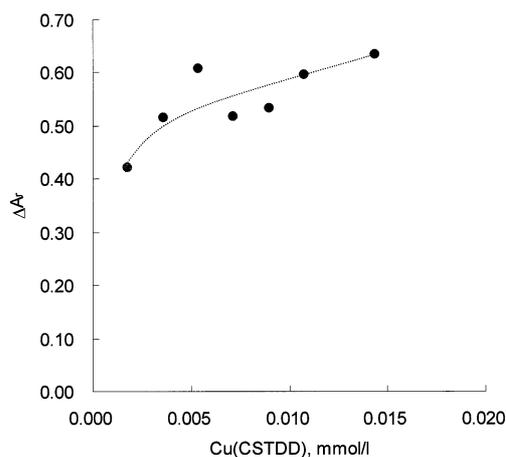
Fig. 8 Effect of molarity of Cu(CSTDD) on  $\Delta A_r$  of Cu(CSTDD)-Co(II) in the solution where Co(II) was added at a constant ratio at pH 9.43.
