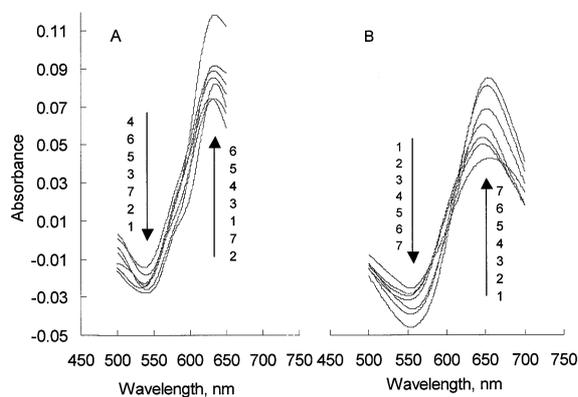
Fig. 1 Effect of pH on absorption spectra of (A) Cu-CSTDD complex in solution containing 0.01435 mmol/l CSTDD and 1.00 mg/l Cu(II), (B) Co-CSTDD complex in solution containing 1.00 mg/l Co(II), with corresponding pH labeled from 1 to 7: 8.13, 8.65, 9.00, 9.24, 9.43, 10.00 and 10.60, respectively.
