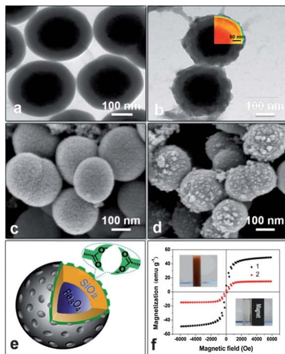
**Fig. 1** TEM and SEM images of Fe<sub>3</sub>O<sub>4</sub>@SiO<sub>2</sub> (a and c), Fe<sub>3</sub>O<sub>4</sub>@SiO<sub>2</sub>IIPs (b and d), cartoon illustration of microsphere (e), and magnetization curves of Fe<sub>3</sub>O<sub>4</sub> (1) and Fe<sub>3</sub>O<sub>4</sub>@SiO<sub>2</sub>@IIPs (2) (f), and digital photographs of the solutions containing Fe<sub>3</sub>O<sub>4</sub>@SiO<sub>2</sub>@IIPs before and after magnetic separation with the help of an external magnetic field (inset).
