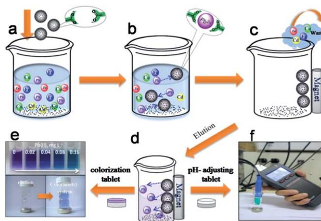
Fig. 3 Preconcentration and onsite monitoring of lead in water samples with  $\text{Fe}_3\text{O}_4@\text{SiO}_2@\text{IIPs}$ : adding the extractants (a), selective adsorption (b), magnetic separation (c), elution (d), onsite colorimetric determination (e) and onsite electrochemical determination (f).
